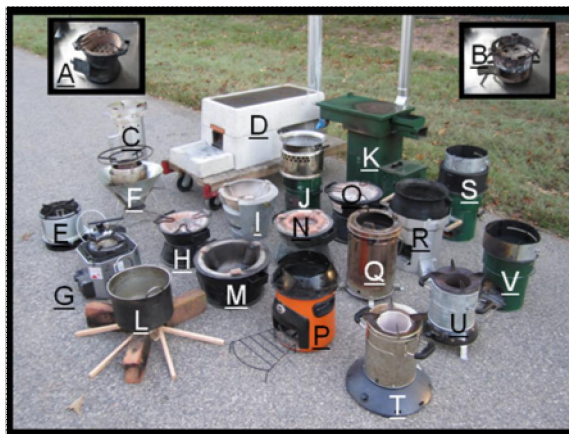
Figure 1. Stoves Tested: A. Ceramic Jiko, charcoal; B. Metal Jiko, charcoal; C. Belonio, rice hull; D. Onil, wood; E. Protos, plant oil; F. Mayon Turbo, rice hull; G. Oorja, pellet; H. KCJ, charcoal; I. GERES, charcoal; J. StoveTec, charcoal; K. Jinqilin CKQ-80I, corn cobs; L. 3-Stone Fire, wood; M. Upesi, wood; N. Uhai, charcoal; O. Gyapa, charcoal; P. Envirofit G-3300, wood; Q. Sampada, wood; R. Berkeley Darfur, wood; S. StoveTec TLUD, pellet; T. Philips HD4012, wood; U. Philips HD4008, wood; V. StoveTec, wood.
